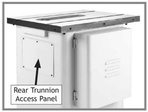
**Figure 95.** Location of the rear trunnion access panel.
